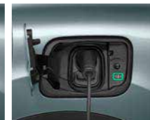
Charging Mode in Progress (Flashing green LED)
