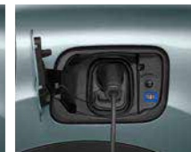
Deferred Charge Mode (Flashing blue LED)
